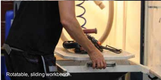
The DC Box is a specially designed dust extraction cabinet that protects against hazardous dust during decontamination and cleaning before servicing or repairing machines and tools. The DC Box is equipped with a blow gun and a suction hose for vacuum cleaning. Larger particles and debris fall down into a plastic bag attached to the bottom of the cabinet.
