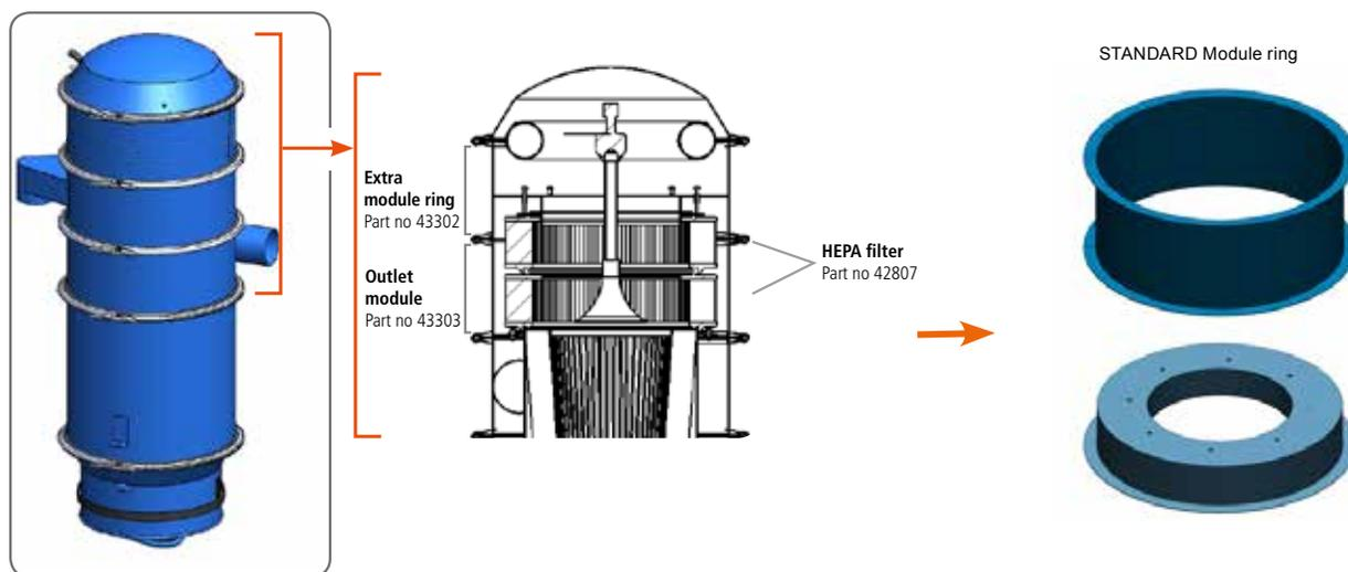
S11000 filter units, DC 11000 dust extractors and DC 11-modules may be combined or completed with Dustcontrol's HEPA-Module. It fulfills the HEPA H13 specifications and is excellent for cleaning air. The module is specially suited to capture the smallest and most dangerous particles. It also works as an extra protection for the pump and motor.
