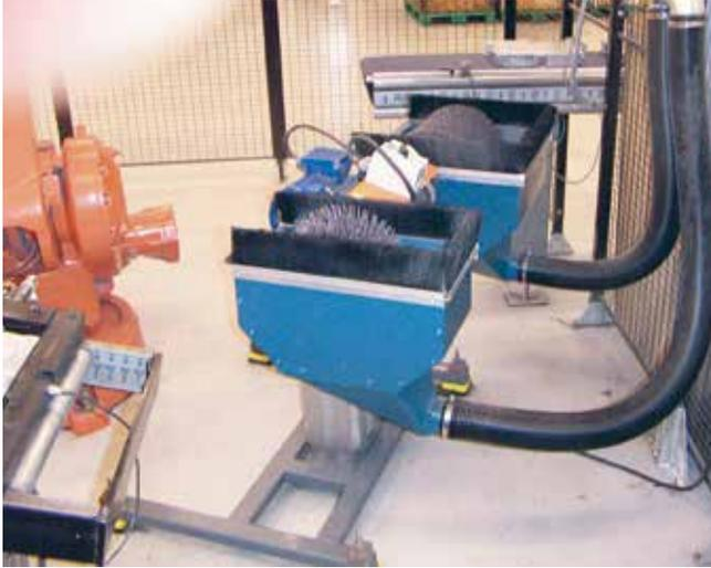
Robot deburring for telecom parts
