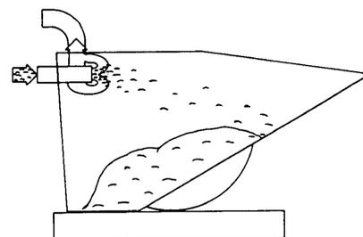
**Inertial Principle** meaning that the air stream flows into the container and abruptly changes course.
