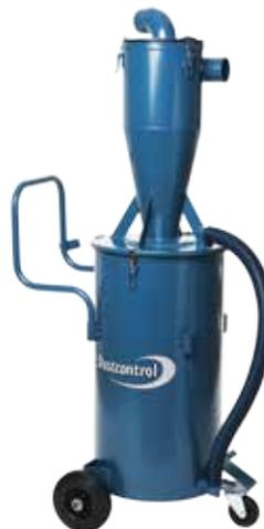
The DCF Mobile Cyclone has a high efficiency cyclone mounted on the top cover. Thanks to the small diameter of the cylinder in relation to its height and to the specially shaped inlet, this separator can separate even smaller and lighter materials such as asbestos fibres. The separated material then falls into the container which is fitted with a plastic bag for dust-free handling.
