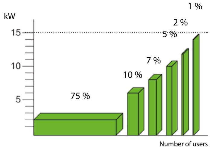
With a 15 kW vacuum producer with DC Green System the rpm and energy use is matched with the number of people using the system at the same time.
