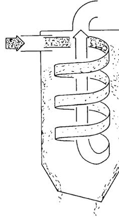
**Cyclone Principle** meaning that the inlet is mounted tangentially on the body and the air flow is thus forced against the inside of the cyclone.
