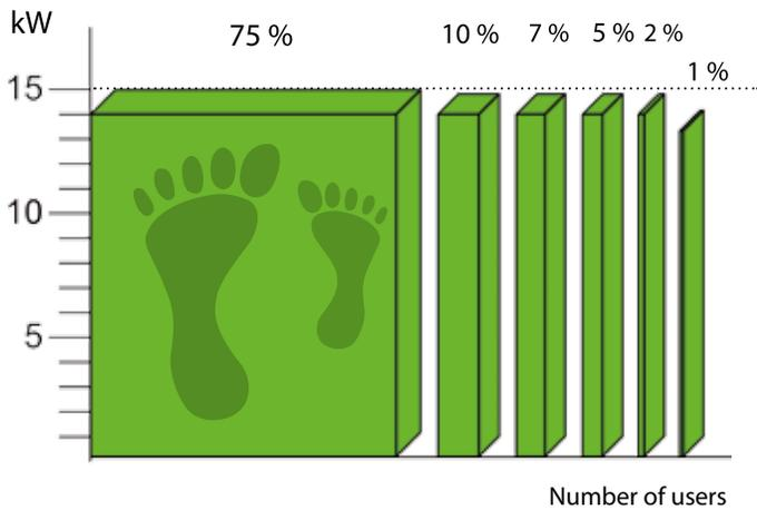
With a 15 kW vacuum producer and a traditional vacuum system, the rpm is almost constant, no matter if the entire plant is using the system or if one employee is using the system.
