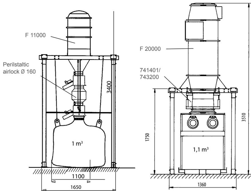
F 20000 with widening chassis and discharge into a 1.1 m<sup>3</sup> container.
